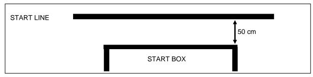
The start line and start box are marked at the start. The start beam is located at the Start Line. The start box is positioned 50 centimetres behind the start line.
